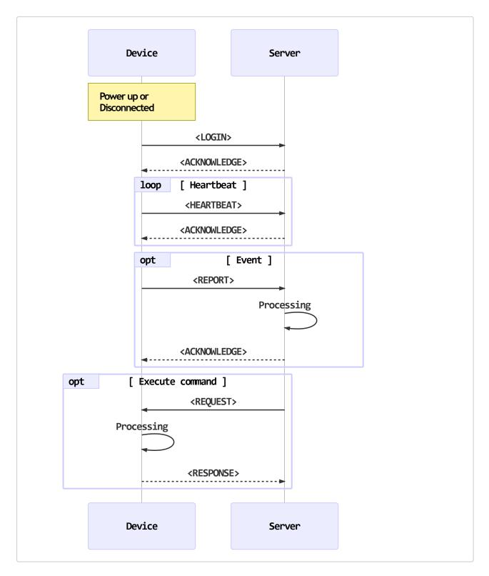
When device is powered up or session is disconnected, it attempts to establish a connection to server. After being connected, device sends a login package to server at first. All other packages will not be sent until device received the acknowledge from server.
